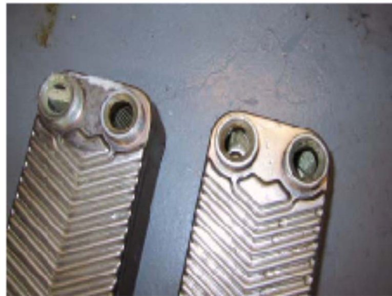
Fig. 6. Comparison photo of the flow channels of the "baseline" heat exchanger (LHS) and the heat exchanger equipped with the passive back flow system (RHS) at the end of the testing period.
