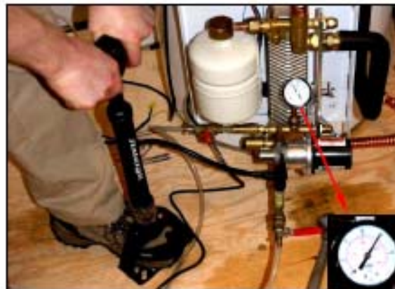
Fig.5.1.2 – Leak-test: pressurize appliance to 40 psi and wait 30 minutes.
