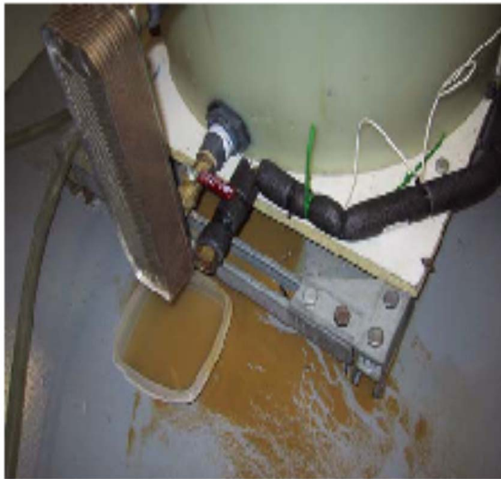
Fig. 5. Photo of the "baseline" heat exchanger at time of removal from the test rig.
