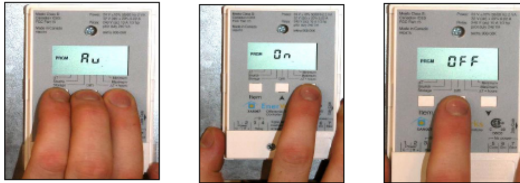
Fig.5.3.2 – Manually start pump by pushing all three buttons to enter program (PRGM) mode then push down button. To shut off, enter PRGM mode and push up button.
