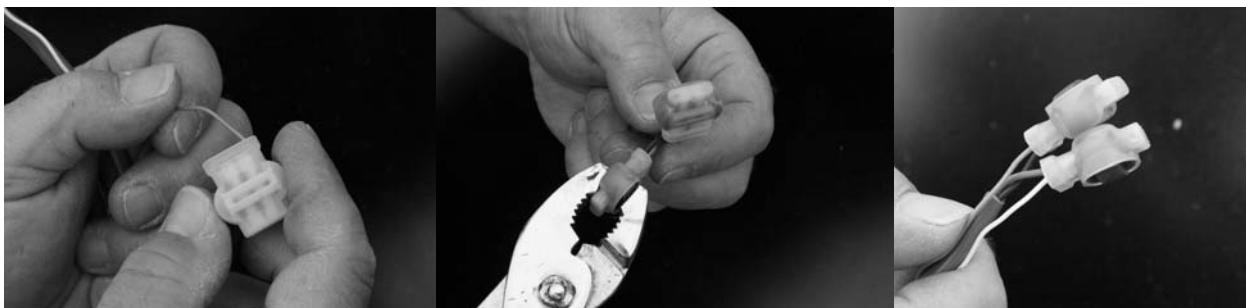
Fig. 6.4.1 – To make thermistor/control-wire connections, insert unstripped conductors into IDC and squeeze with pliers.
